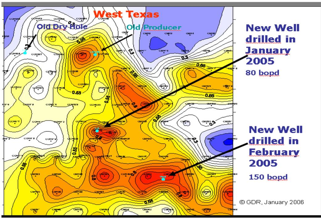
Fig. 2 Detection and mapping of spatial and depth distribution of hydrocarbon accumulations in West Texas. Red to yellow figures represent oil accumulation zones where isolines represent net oil pay zone thickness; whereas blue figures present water-saturated zones (See color scale captions in Fig. 8, which represents direct hydrocarbon indicator, as function of cumulative net oil pay zone thickness)
